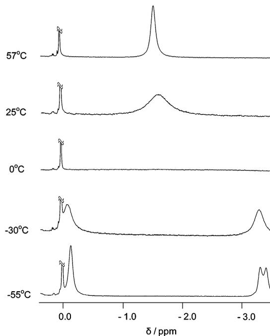
**FIGURE 4.** Section of the methyl signals of the guest in the <sup>1</sup>H NMR spectrum (CDCl<sub>3</sub>, 400 MHz) of [**10b**·Et<sub>4</sub>N<sup>+</sup>·**10b**] PF<sub>6</sub><sup>−</sup> at different temperatures.
