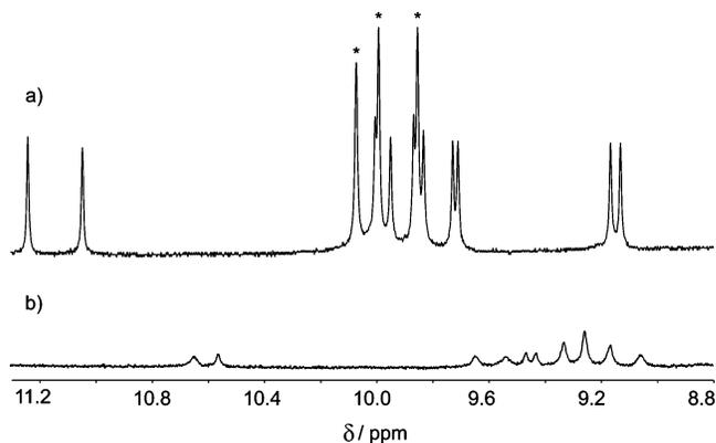
**FIGURE 2.** Section of the  $^1\text{H}$  NMR spectra of a mixture of **10b** and **13a** (ratio 1:1.1) in (a) benzene- $d_6$  and (b)  $\text{CDCl}_3$ . Low field signals for 16 protons (peaks marked by an asterisk have the double intensity) indicate the formation of two regioisomeric heterodimers (two times eight  $-\text{NH}_\alpha-$  groups) in nearly equal quantity (a).
