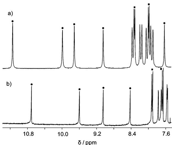
**FIGURE 3.** Section of the <sup>1</sup>H NMR spectra of a mixture of **10a** and **14** (ratio 1:1.1) in (a) benzene-*d*<sub>6</sub> and (b) CDCl<sub>3</sub>. Assignment of peaks: filled circles, N–H (5 or 4 of 7 singlets); filled squares, tolyl Ar–H (2 of 4 doublets); remaining peaks, calixarene Ar–H.
